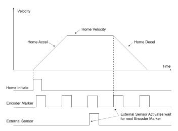
Figure 37: Home to Sensor then Marker Profile (Calculated Offset)
